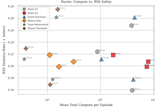
Fig. 6. Mean total compute vs. RSS violation rate across 3 highway-env scenarios \times 6 methods. TM-C (star markers) occupies the low-compute, low-violation region in all scenarios.
