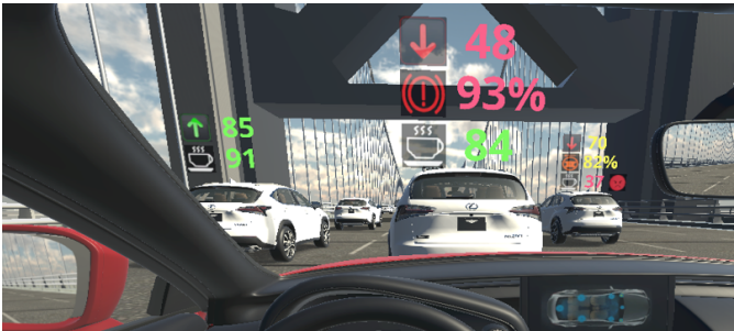
Fig. 6. Prediction and guidance information received from the Vehicle Digital Twin on the cloud is visualized through an augmented reality (AR) head-up display (HUD), which may include: driving proficiency score and its trend, potential action (e.g., hard braking or lane change) and its possibility, as well driving mood score.
