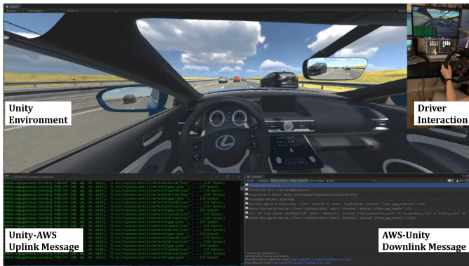
Fig. 5. Human-in-the-loop simulation of the cloud-based ADAS based on AWS, the Unity game engine, and the Logitech G29 Driving Force.
